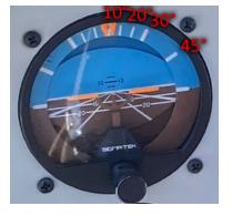
self-correcting instrument, and as the gyroscope *precesses* (is affected by friction), it makes small corrections to remain upright.
