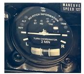
rate of turn of 3 degrees per second. When turning at this rate, the airplane will make a full 360 degree turn in 2 minutes. This is called a *standard rate turn*, and is used for all turns in instrument conditions.
