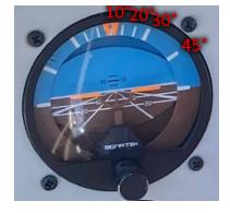
self-correcting instrument, and as the gyroscope *precesses* (is affected by friction), it makes small corrections to remain upright.
