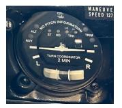
rate of turn of 3 degrees per second. When turning at this rate, the airplane will make a full 360 degree turn in 2 minutes. This is called a *standard rate turn*, and is used for all turns in instrument conditions.
