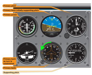
Roll Out of Turn - Begin to gently reduce bank 10-20 degrees before target heading to avoid overshooting the turn. Re-establish level flight by using the attitude indicator to level the wings.
