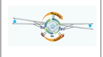
Spiraling Slipstream - As the airflow moves through the propeller and around the fuselage, wings, and control surfaces, it is spinning. The spinning propeller imparts a considerable spiraling motion to the slipstream, and because the vertical tail surface extends only above, and not below, the spiraling slipstream pushes the tail slightly right, leading to left yaw.
