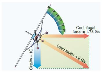
As the bank angle increases, the load factor required to maintain level flight increases slowly at first, but increases rapidly, especially at bank angles beyond 45 degrees. The load factor
