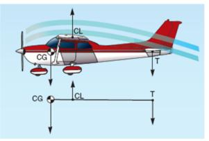
This design causes a natural tendency for the airplane to nose down, reducing the angle of 0 attack. To counteract this, the horizontal stabilizer and elevator surfaces of an airplane are designed to produce a *downward* force, which 'holds up' the heavier nose area by pivoting the airplane around the Center of Lift. When an airplane stalls, if the elevator pressure is relaxed, the Center of Gravity will fall naturally.
