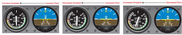
To maintain straight and level flight, pilots should scan between the attitude indicator, and the primary pitch, bank, and power instruments: the altimeter, directional gyro, and airspeed indicator.
